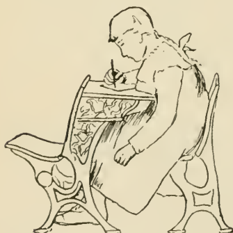
FIG. 41. — Illustrating a too small distance between the seat and desk, causing pressure on chest and stomach.
